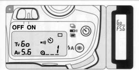
\* When the shutter release button is depressed halfway down, the shutter speed and aperture value will be displayed in the viewfinder and on the LCD panel. The bar underneath the shutter speed indicates that you can change the shutter speed.
