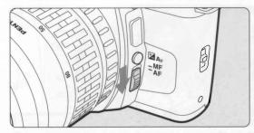
For autofocus operation, set the focus mode switch to [AF]. When you depress the shutter release button halfway down, the lens automatically focuses.
