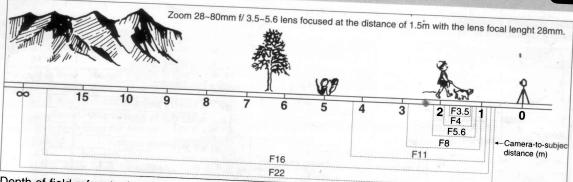
Depth of field refers to the range around the optimum focusing point of the subject in which the elements at different distances are in focus. The depth of field increases as the aperture is closed down, the focal length of the lens becomes shorter, or the subject is positioned farther away.
