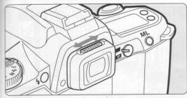
Aim the camera at a bright subject. While looking through the viewfinder, move the diopter adjustment lever to the left or right until the autofocus frame [ ] appears in the sharpest focus.
