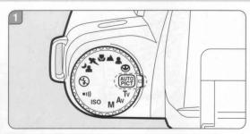
This Auto Picture Mode allows you to take pictures by simply depressing the shutter release button. In this mode, the camera automatically selects one of 5 picture modes according to the requirement of the scene.
