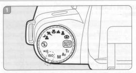
This camera automatically reads the film speed from the film's DX code. However, the film speed setting can be changed. If you use a non-DX coded film, set the film speed manually.
