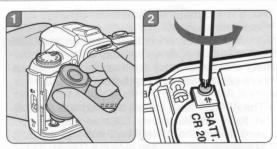
Replace the battery when the data information on a picture or the LCD panel becomes weak or invisible. The battery will last for approximately 3 years. The data back uses one 3V lithium battery, type CB2025.
