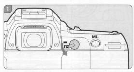
You can switch between the panorama format and standard format picture taking mode in the middle of the roll by moving the panorama lever. The panorama format picture allows horizontally positioned dynamic pictures to be taken (the panorama format is approximately 13x36mm on the film).
