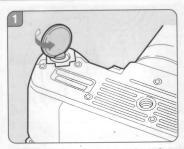
Open the battery chamber cover by using a coin, etc. as shown in the illustration.
