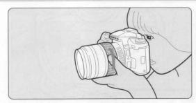
Turning the zoom ring to the right makes the subject appear larger (telephoto) and turning it to the left makes the subject appear smaller (wide angle).
