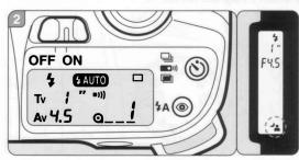
\* When the shutter release button is depressed halfway down, [-1\_a] is displayed in the viewfinder. The shutter speed and aperture setting are also displayed in the viewfinder and on the LCD panel.
