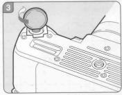
Turn the battery chamber cover screw in the direction of the arrow to lock it securely.
