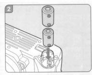
Load two 3V lithium batteries (CR2) or equivalent as shown in the illustration.
