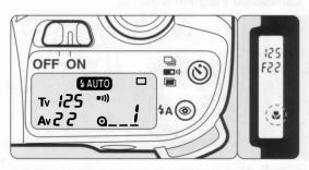
This mode is useful for close-up photography. This mode favors smaller apertures to maximize the depth of field, ensuring sharp focus of a close-up subject.
