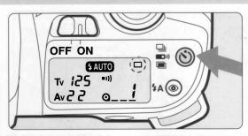
Depress the drive button until [□] appears on the LCD panel.
